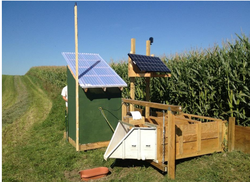
Edge-of-field monitoring stations help to evaluate agricultural runoff and its impacts to water quality.
