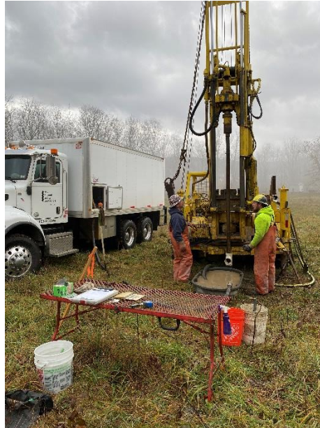
Stone staff advance soil borings in support of wastewater disposal site capacity determination (left). The Trout River (right) is being sampled at two locations in Montgomery Center in support of Indirect Discharge permitting.
