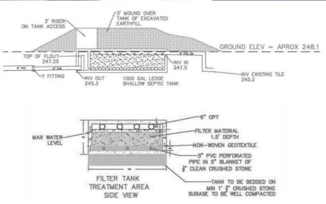
Details extracted from construction drawings of the subsurface tile drain treatment system designed, installed, and operated by Stone on a Franklin County farm.
