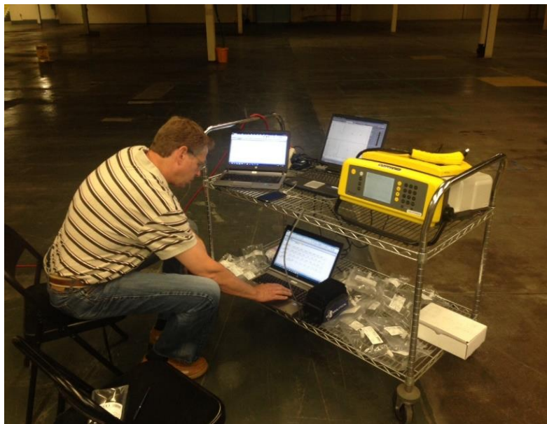
On-Site analysis of air samples at the former Energizer facility in St. Albans, Vermont using a field portable gas chromatograph/mass spectrometer.
