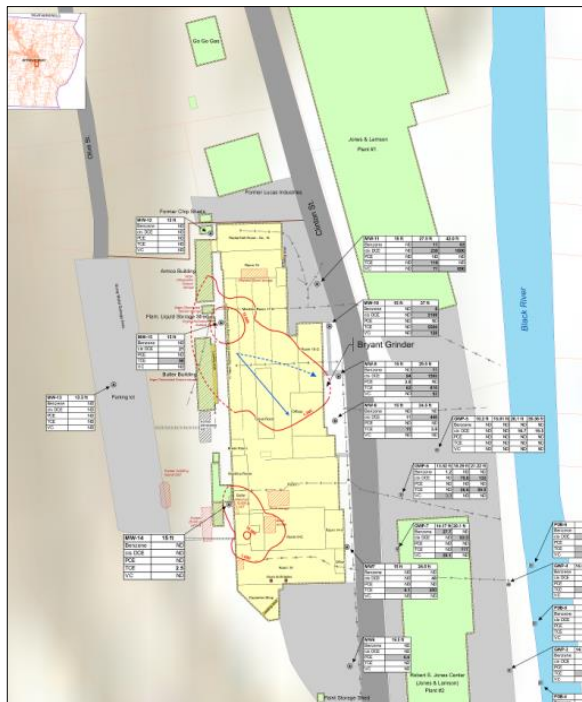
The Membrane Interface Probe provided real-time data to assess plume cores along the downgradient property boundary.
