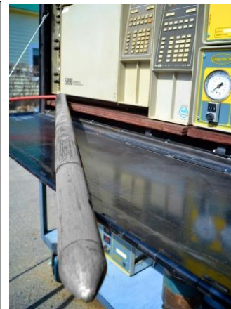
The Membrane Interface Probe provided real-time data to assess plume cores along the downgradient property boundary.
