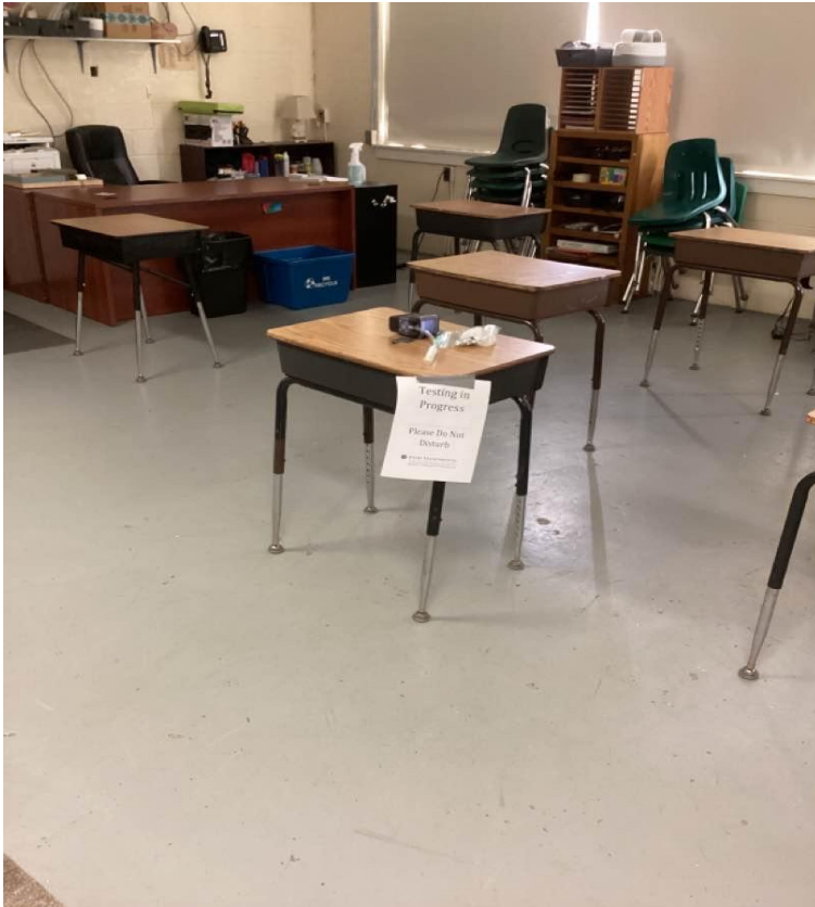
Typical air sample pump and cartridge for PCB air testing in schools
