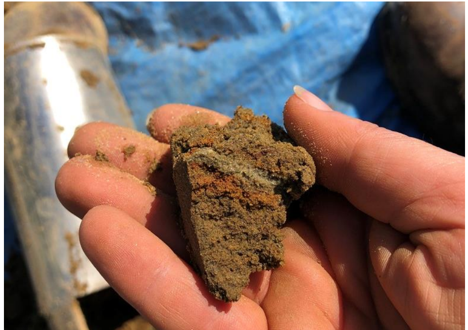
Site-specific soil evaluation throughout the Helen Ave. drainage revealed sandy soils and shallow groundwater.
